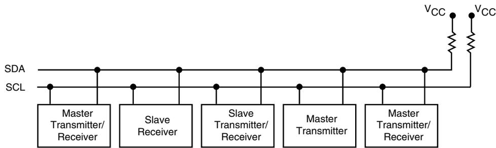
**Note:** Due to open drain configuration of SDA and SCL, a bus-level pull-up resistor is called for, (typical value = 4.7k $\Omega$ )
